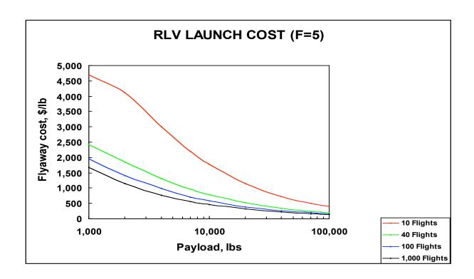
Figure 4. Flyaway cost versus payload size and vehicle lifetime for a fleet of 5 RLVs.
