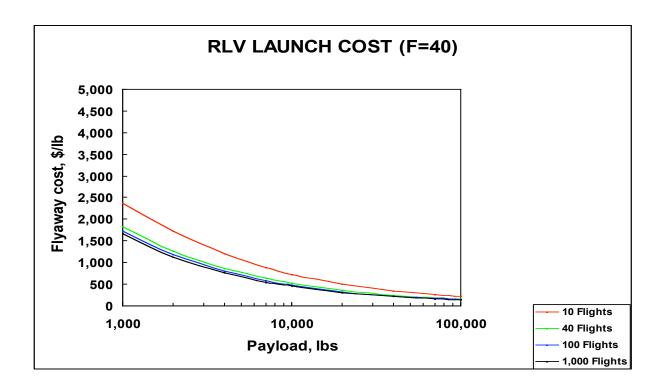
Figure 5. Flyaway cost versus payload size and vehicle lifetime for a fleet of 40 RLVs.
