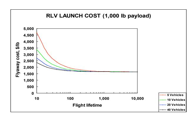
Figure 2. Flyaway cost versus vehicle lifetime and fleet size for 1,000 pound payloads.
