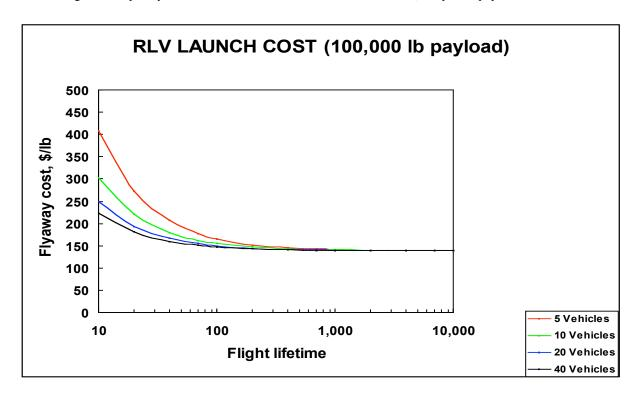
Figure 3. Flyaway cost versus vehicle lifetime and fleet size for 100,000 pound payloads.
