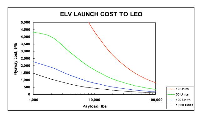
Figure 1. Flyaway cost per pound to LEO versus payload size and production run for a 10 year program.
